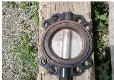
Fig. 7. Damper in disassembled form after heating season with device
